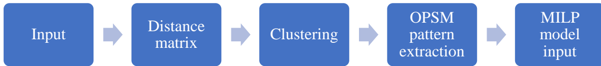
Figure 2. Flowchart of Optimal Facility Location Process Using Clustering and MILP
