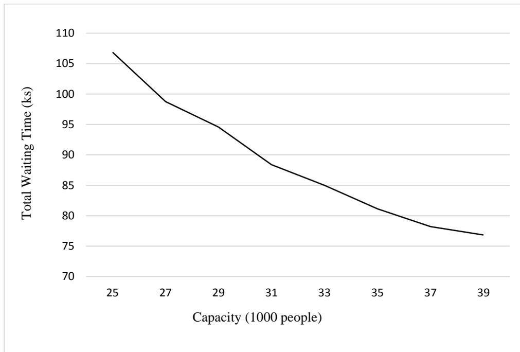
**Fig. 1.** Effect of Trains' Capacity on Total Waiting Time
