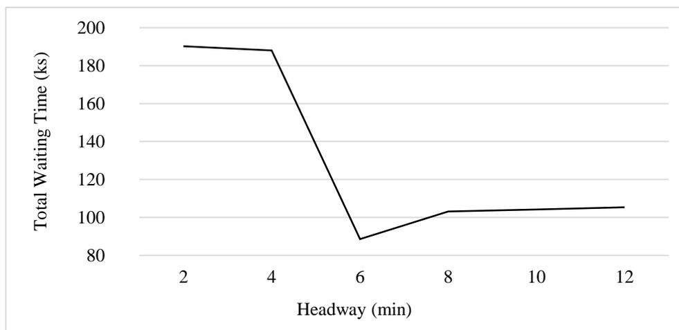
**Fig. 3.** Effect of Headway on Total Waiting Time
