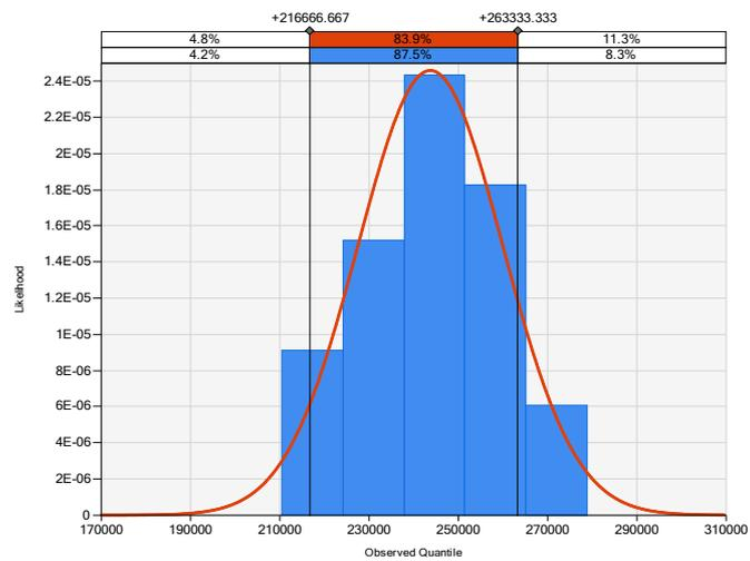
**Fig. 3.** Probability Density Function of Demand Load (PDF)
