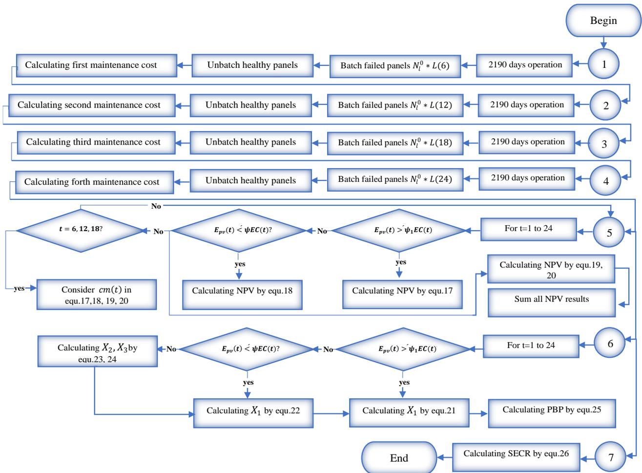
Fig. 5. Simulation process in scenario I
